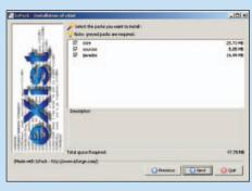
Figure 2 • eXist installation step 2. If you are going to do Java development, you should select "javadoc"; if you are interested in eXist sources, select "sources" too.
